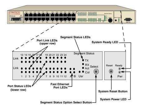
Figure 6-1 FN10 Front Panel LEDs
